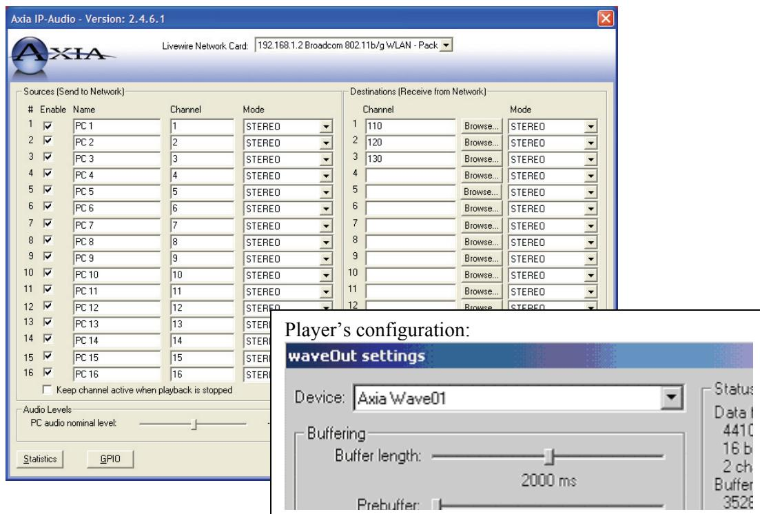
Axia Element or SmartSurface consoles will use this source, so a Source Profile must be configured, as shown below (See the Element or SmartSurface users manual for instructions on how to construct a Source Profile).
